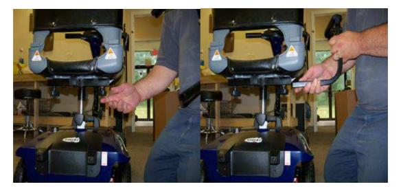
• Set the armrest to the desired location and tighten the armrest-locking knob. Repeat for the other side.
