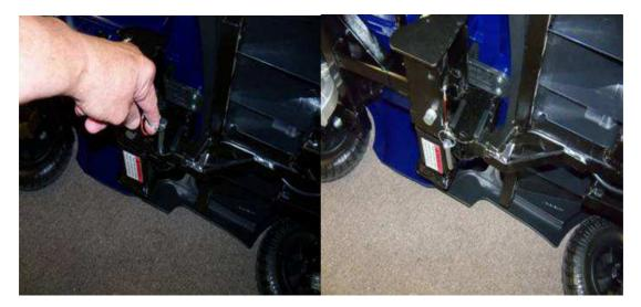
Verify the tiller is locked in place, see step 18. Lift up on the battery box while hold on to the front section of the base. This will separate the front and rear sections. Unlock and remove the battery box. To reconnect the front and rear section, reverse the above steps. The two yellow marks on the front section and the two yellow marks on the rear section must be aligned to reconnect both sections.
