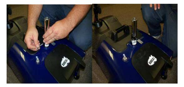
• Install the seat post knob into the seat post receiver and tighten. If the seat height has to be adjusted, loosening the seat post knob and removing the grenade pin can do it. The adjustable seat post then can be moved up or down as needed. Install the grenade pin and tighten the seat post knob.
