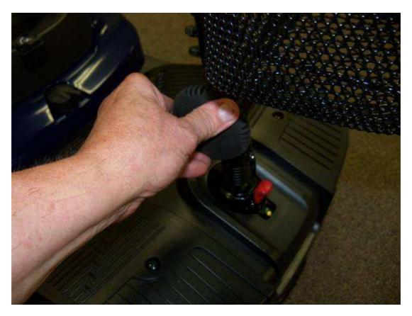
• The Bobcat is shipped with the tiller locked in the straightforward position. To unlock the tiller lift up on the tiller locking lever. The tiller should be locked when lifting up the base or the front section of the Bobcat.
