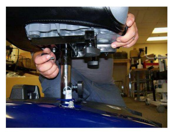
• Loosen the armrest-locking knob and slide the armrest into the seat plate.
