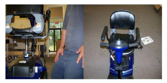
Slide the basket over the basket mounting brackets on the front of the tiller.
