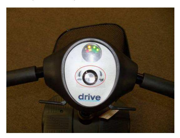
Push the forward side of the throttle lever towards the handle bar to go forward. Push the reverse side of the throttle
