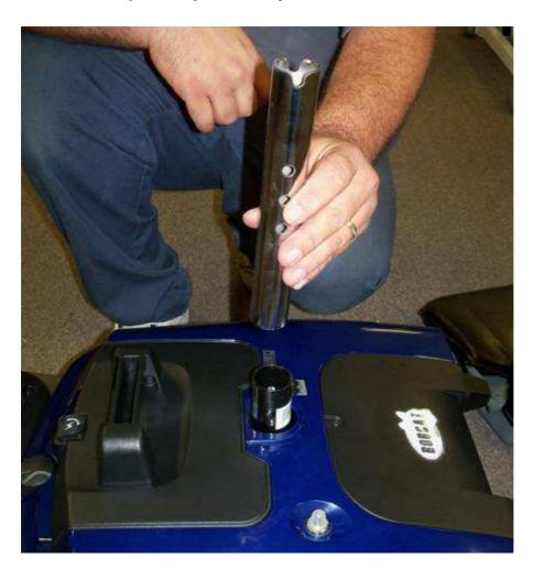
Select a height and install the grenade pin through the base and the adjustable seat post.
