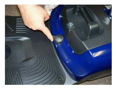
• Remove the battery box by lifting straight up.
