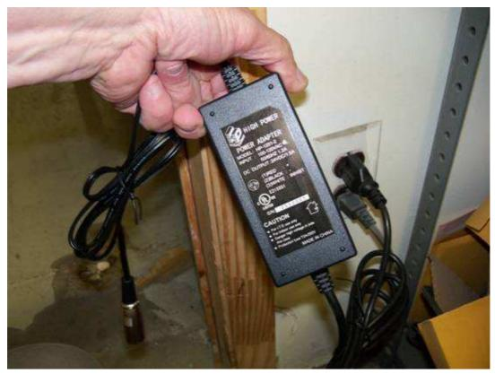
• Plug the charger into the battery pack. The light on the charger will turn red and as the batteries charge the light will turn green when the batteries are fully charge. The battery pack can be charged either on or off the Bobcat.
