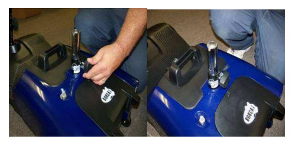
Remove the locking knob off the seat plate seat post receiver and slide the seat unto the seat post.
