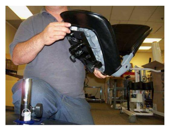
• Install the locking knob back onto the seat plate.
