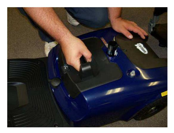
• Remove the protective plastic sheet. Put the battery box back into the Bobcat base and lock in place.
